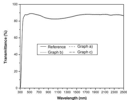
Fig. 4. Transmittance results of the test on soda-lime glass without feeding material.
