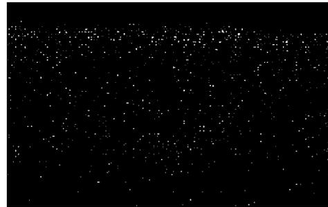
Fig. 2. A carbon mapping on copper obtained by SEM.
