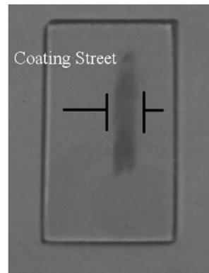
Fig. 3. Soda-lime glass sample coated with iron oxide by triboadhesion.
