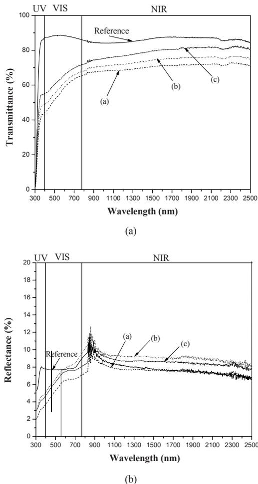
Fig. 5. Triboadhesion test results on a soda-lime glass sample coated with iron oxide by triboadhesion: a) Optical transmittance and b) reflectance. The terms UV, VIS and NIR represent the Ultra Violet, Visible and Near Infrared spectral radiation regions.
